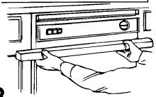
Latch dishwasher door. Push dishwasher into place, sliding drain hose through hole cut in cabinet opening. Do not pinch power supply cord or kink power supply cable between dishwasher and cabinet. Check that front leveling legs are firmly against the floor. Align dishwasher door with cabinet doors, so that spacing is the same on both sides.
